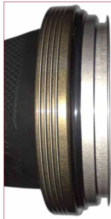
Putting on the sealing o-ring into the slot. The type and measurements are stated in the section: dInstructions for use „Part I.: Description\_maintenance\_service\_solving problems“.
